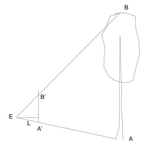
A Merritt hypsometer is a stick marked to measure similar triangles. It is unusually held 25 inches from your eye (L) and allow the tree height to be measured as a ratio of the distance from the tree. This method is usually used to measure large height classes such as number of 8' or 16' logs in a tree (Husch et al., 2003).
